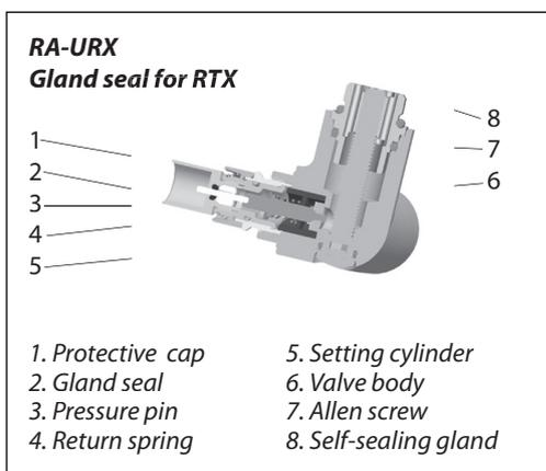
The valve assembly features valve body and a self-sealing gland pre-mounted with 2 O-rings - one for sealing against the radiator and one for sealing in the valve housing.
