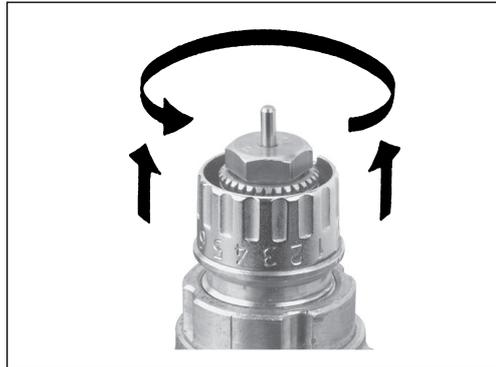
Danfoss pre-settable valve bodies incorporate easy setting adjustment rings with clearly engraved setting markers scaled from 1 - 7 and N. Setting values can be set quickly and precisely, without the need for tools, as follows:
