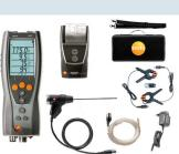
The single integrated flue gas and thermocouple connector of the testo 327 ensures a fast, gas tight connection to the sample hose every time. The testo 327 also has automatic pump protection as standard to help protect the CO measuring cell from damage due to over-range (4,000ppm range capability).
