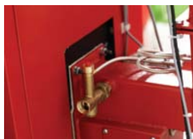
Typical mounting of BVTS when used as back-burning protection
