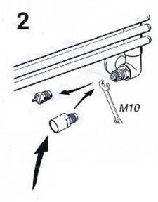
**Attention** The RTX thermostat may only be fitted with the special gland seal enclosed.
