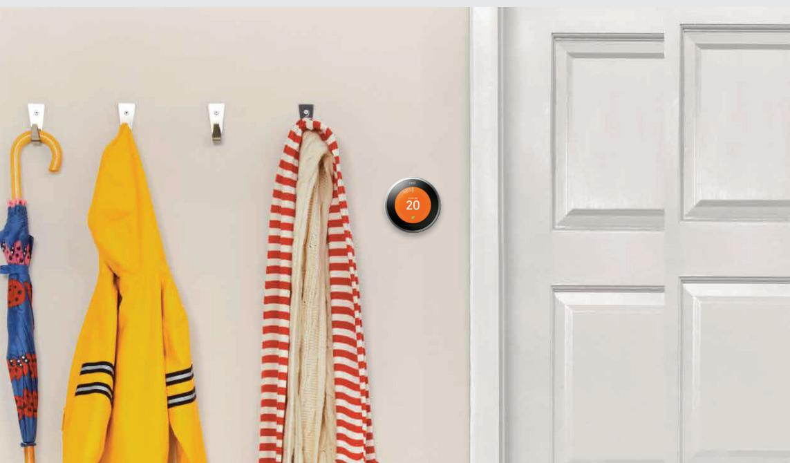
Nest devices. With the geolocation mode selected, Nest will switch to 'Home/Away' mode and adjusts itself to an Eco-Temperature after you leave so you don't heat or cool an empty home. Nest uses two methods for this, your phones location, and a motion detector on the front of the Nest. The combination works brilliantly and should help you save money on heating bills.
