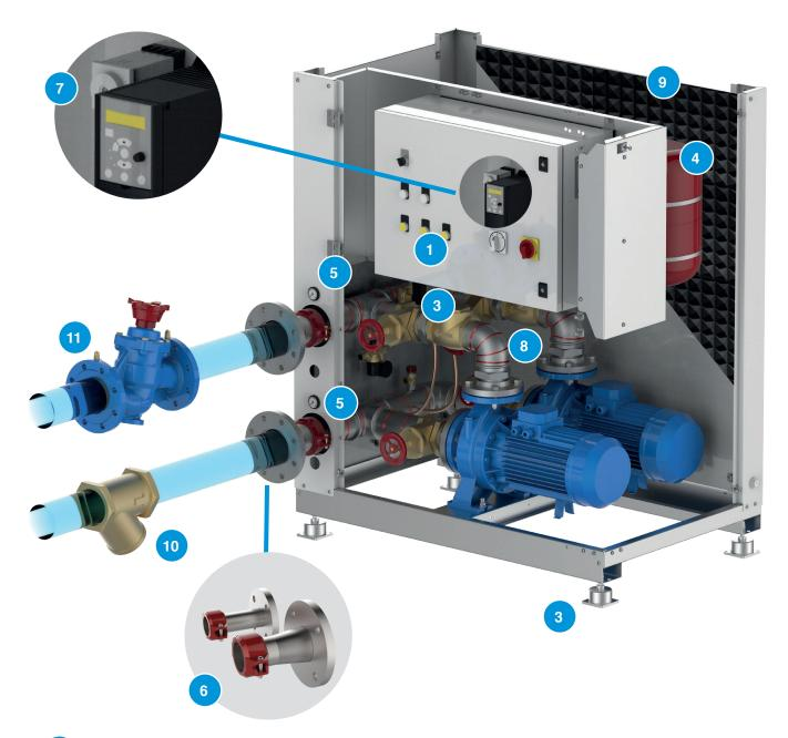
7 Inverter (special version) Each pump can be operated by an inverter. The units equipped with inverters have a pressure sensor, 0-10 bar, which communicates with the inverter with 4-20 mA signal. All adjustment parameters are pre-loaded during the test run at the company. The user must choose only the desired set point pressure value.
