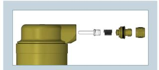
It is possible to rotate the air vent valve through 360° to position the drain appropriately, without needing to shut down the system.
