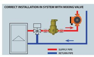
Bubbles mostly appear in the boiler on the surface separating flow and combustion chamber where there are high temperatures. As specified by Henry's Law, at certain values of pressure and temperature there is a certain concentration of gas dissolved in water. Any changes in temperature and pressure may cause the concentrations of dissolved gases to vary.
