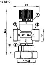
If the thermostatic mixer is installed on a fix point regulating unit for under floor heating system, the temperature value is readeable on the thermometers of the unit. Once fixed the handle position of the mixer, the system is regulated.
