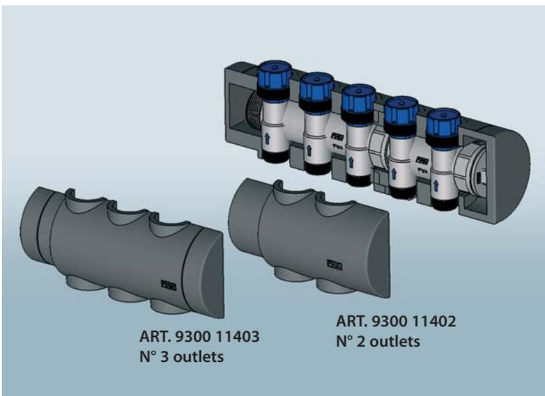
PPE pre-formed anti-condensation insulation can be used to thermally isolate manifolds. Insulation is available for modular 2, 3 and 4 port manifolds and must be assembled in the box after manifold installation.
