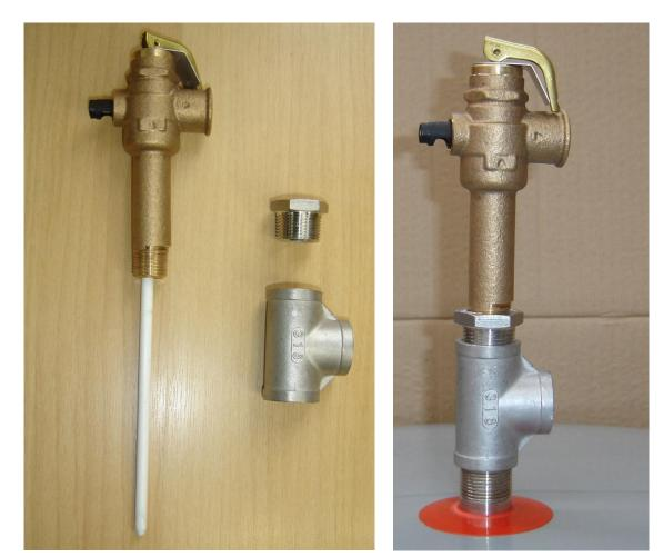
Reliance 850kPa, 99°C TPR kit supplied with the 200 and 300 litre single coil cylinders. May need to fitted before siting the cylinder if headroom is limited.
