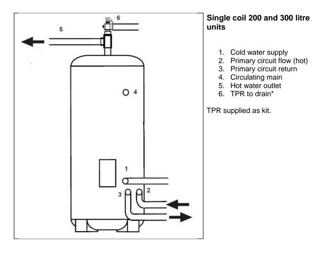
A ring main can be installed on the sanitary water circuit. A connection is provided for the recirculation circuit return pipe (threaded  $\frac{1}{2}$  " female). This connection is supplied with a blanking plug fitted.
