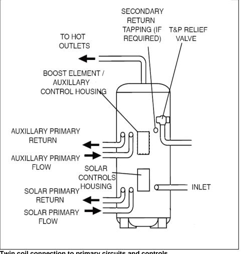
Twin coil connection to primary circuits and controls.
