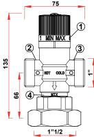
If the thermostatic mixer is installed on a fix point regulating unit for under floor heating system, the temperature value is readeable on the thermometers of the unit. Once fixed the handle position of the mixer, the system is regulated.
