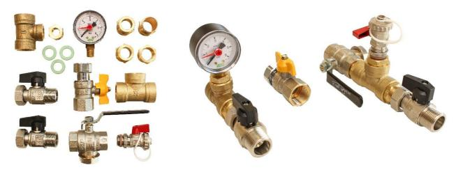
The **BRIFS** fitting kit is specific to the Rinnai I-Series boiler. This kit is intended to make the straight connection of primary feed pipes and gas as simple and compact as possible and still retain key components such as a filter/strainer, drain/fill valve, pressure gauge and ball valves with gasketed swivel unions for ease of connection.
