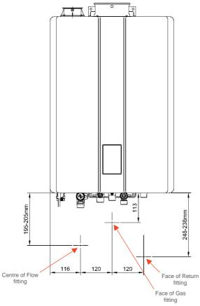
To achieve the dimensions stated above it is recommended that all fittings are threaded as close to the bottom threads where possible. CHNZ recommend using Loctite 55 thread cord, Hemp and Hawk White or other thread sealing products for these joints.
