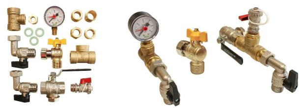
The **BRIFA** fitting kit is specific to the Rinnai I-Series boiler. This kit is intended to make the right angle connection of primary feed pipes and gas as simple and compact as possible and still retain key components such as a filter/strainer, drain/fill valve, pressure gauge and ball valves with gasketed swivel unions for ease of connection.
