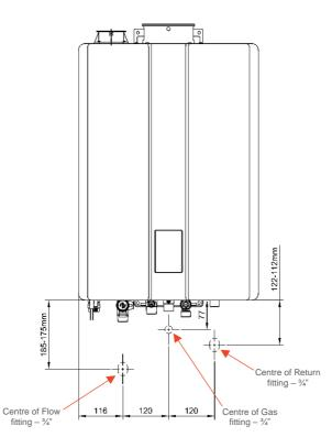
To achieve the dimensions stated above it is recommended that all fittings are threaded as close to the bottom threads where possible. CHNZ recommend using Loctite 55 thread cord, Hemp and Hawk White or other thread sealing products for these joints.
