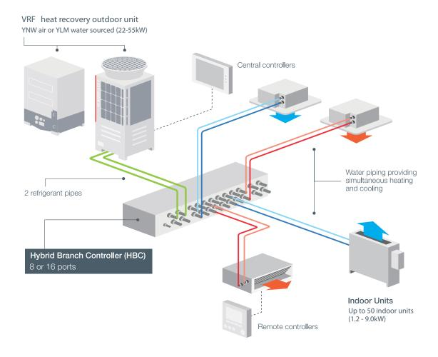
The equipment components suggested will allow you to make the required connections at the HBC box and fan coil.
